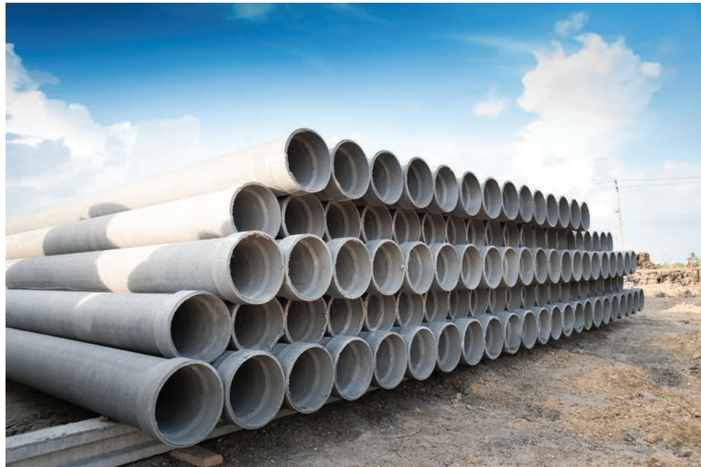
Asbestos cement water pipes were widely used in the 1940s and are used today because of their light weight and supposed durability.
