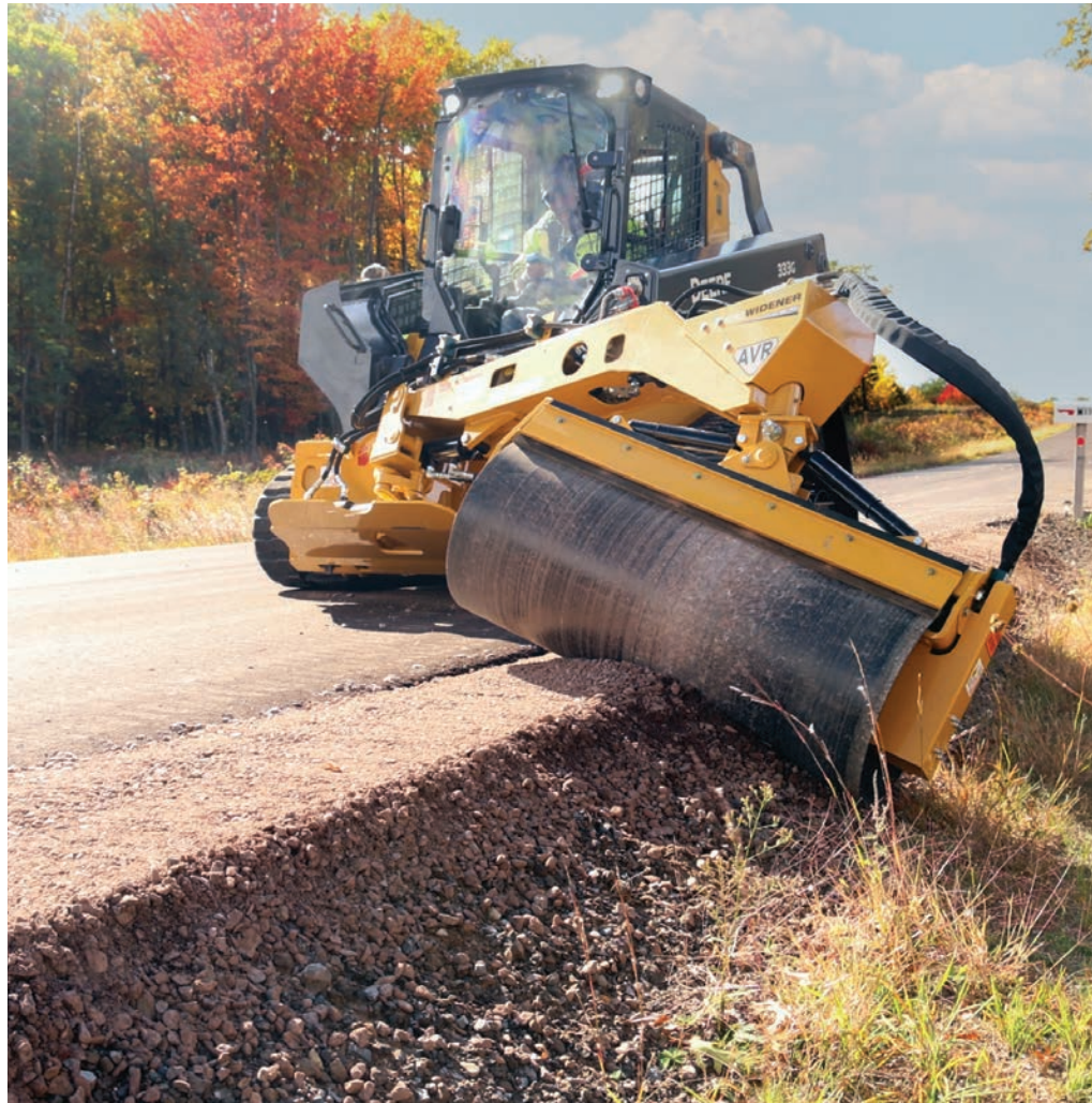
Material placement and offset vibratory rollers are a new generation of attachments that go beyond traditional material loading and digging to create innovative jobsite solutions, improving efficiency and safety. Photo courtesy of Road Widener LLC.
